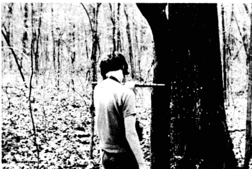
Figure 3. Procedure: A) Holding the "reach stick" at arm's length with the left edge lined up with the left side of the tree, read the diameter size class.
