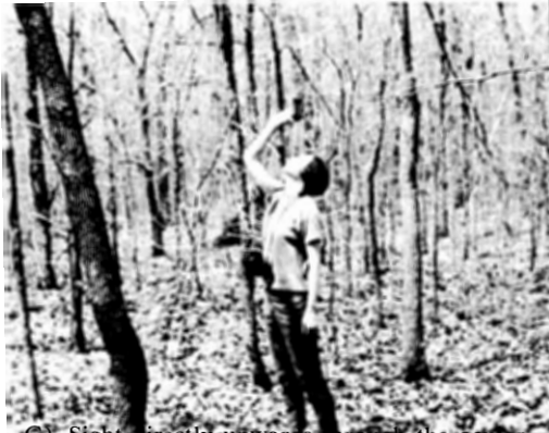
C) Sight directly upwards through the ocular tube to determine the presence or absence of canopy cover.
