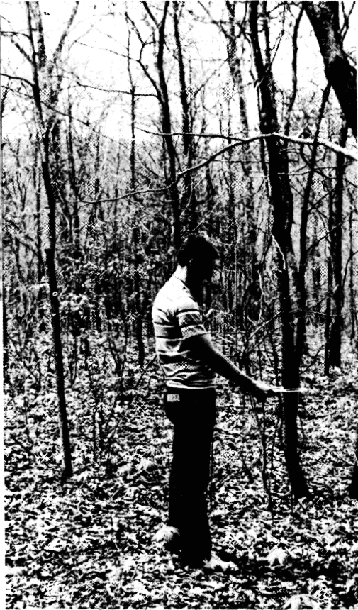
E) Holding the mirror level, walk toward a tree until the crown appears in the mirror. Three feet plus the distance from the mirror to the tree equals the height of the tree.
